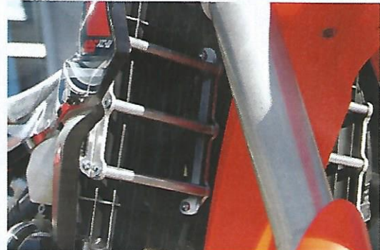
Fix the plastic with M6x16 + M6x20
