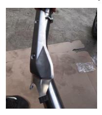
3. Remove the part bracket for silencer with rubber from the tank, and mount it on the DVR silencer as shown on the picture .
